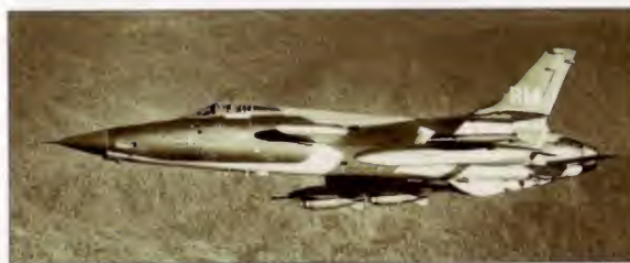
Above: This 355th Tactical Fighter Wing (TFW) aircraft carries a load of M117 and Mk 82 bombs, some with extended fuses.
